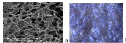
Fig. 3. SEM (a) and optical (b) images of a scaffold after 30 days of fibroblast culture.
