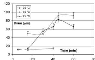
Fig. 2. Pore size of PLLA scaffolds vs. time and temperature
